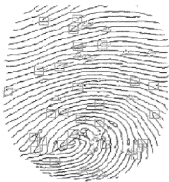
图5 细化图像提取特征点 Fig. 5 Extracted feature points of thinned image
