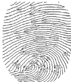
图6 去伪后的细节特征点 Fig. 6 Feature points after removing pseudo-feature
