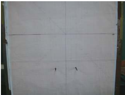
图 4 模拟 2 发弹丸同时着靶装置 Fig. 4 Experimental figure of two projectiles passing through detection area at same time
