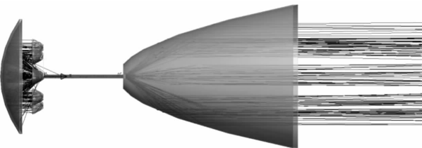
图 8 LED 太阳模拟器模型图 Fig. 8 Model of LED solar simulator
